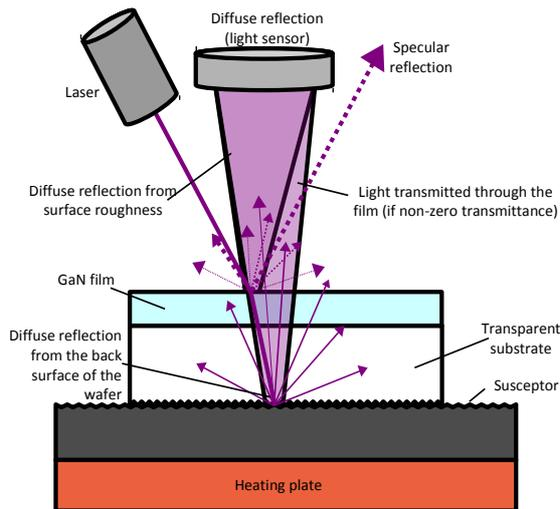
**Figure 2: YGM-BandTime schematic diagram**
