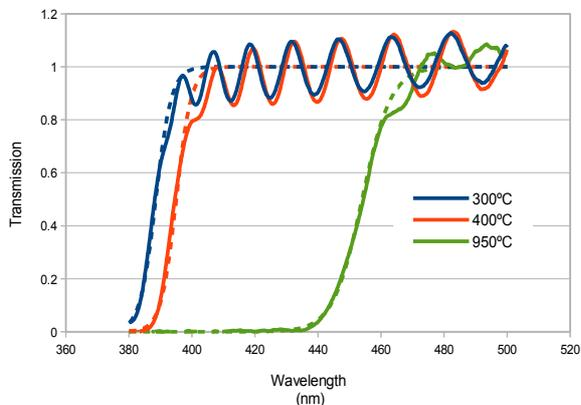
**Figure 3: Temperature dependence of the GaN transmission spectrum**
