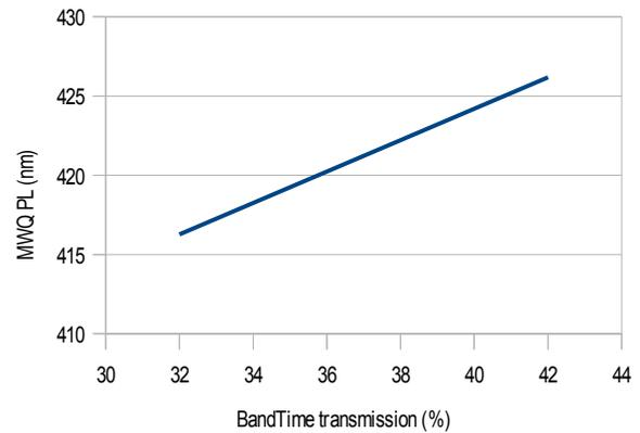
**Figure 6: MQW PL trend vs GaN transmission band-edge @ 445nm**
